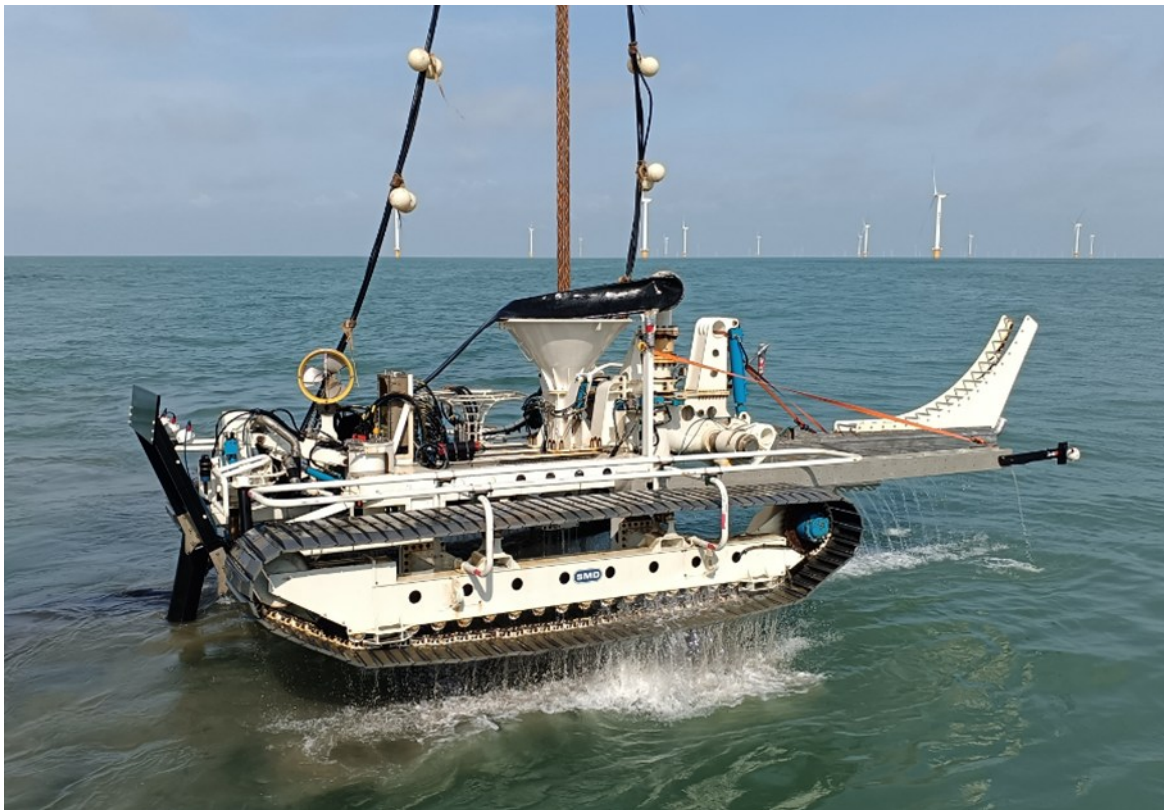
Figur 3.13 Lavvandsgravemaskine (Shallow Water Trencher) (kilde: https://www.smd.co.uk/blog/may-2023-smds-shallow-water-trencher-the-story-so-far/ )
